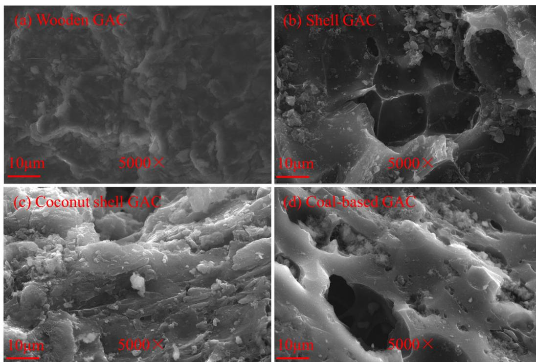
Fig. 1. SEM images of four types of GACs. (a) Wooden GAC; (b) Shell GAC; (c) Coconut shell GAC; (d) Coal-based GAC.
