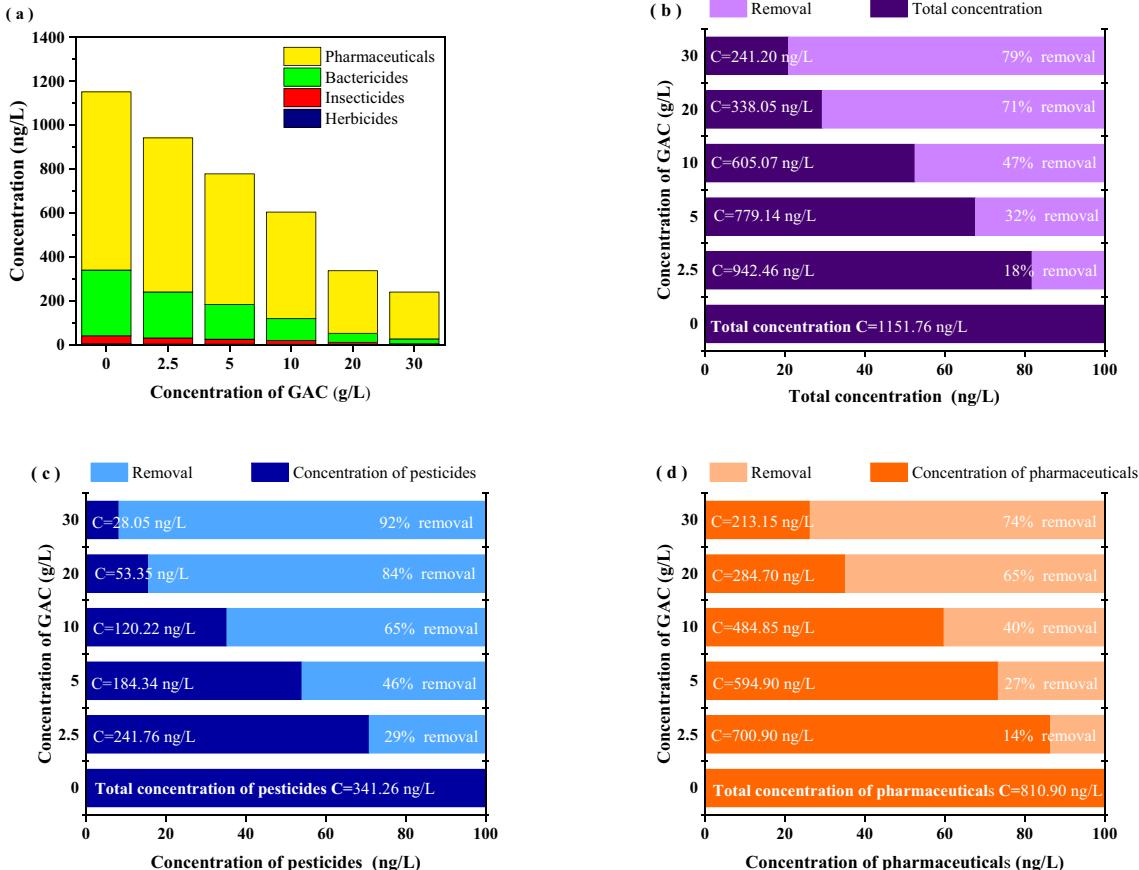
**Fig. 5.** Removal of TOPs by different doses of shell GACs.
