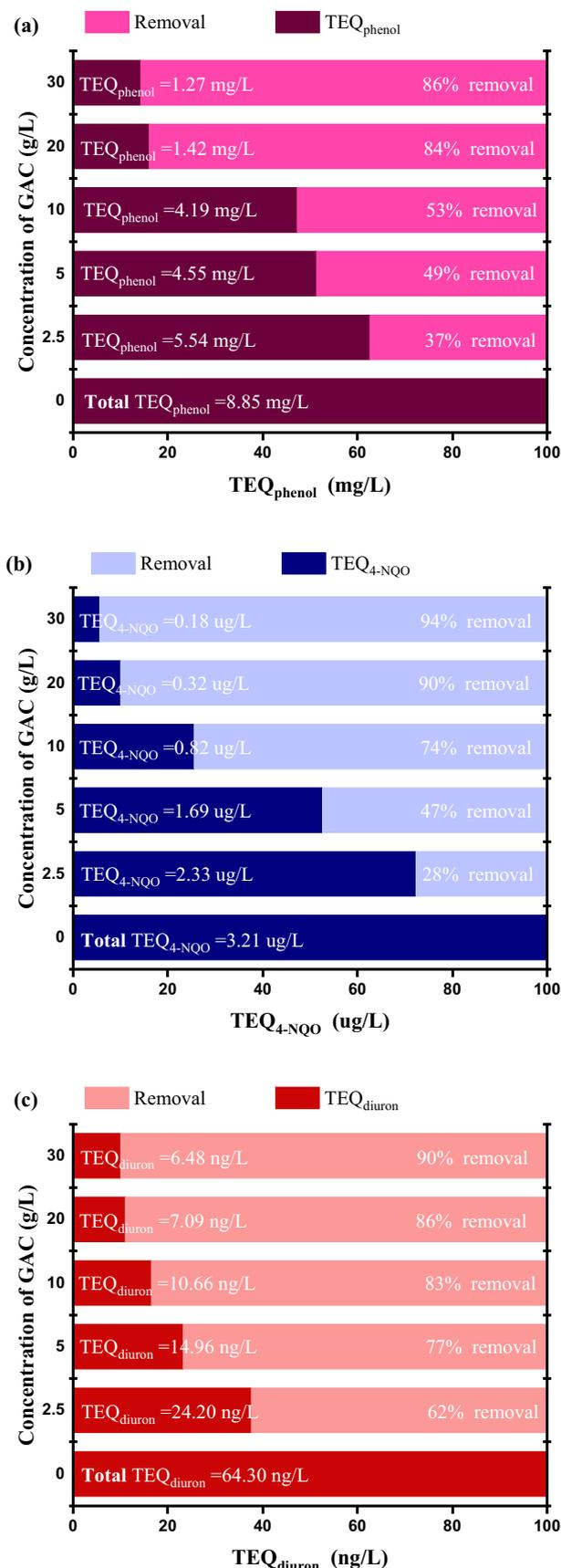
Fig. 6. Removal of three biological effects by different doses of shell GACs. (a) Luminescent bacteria toxicity; (b) genotoxicity; (c) photosynthetic inhibition effect.
