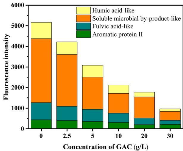
Fig. 4. Fluorescence intensity of four components in wastewater with different doses of shell GAC treatment.
