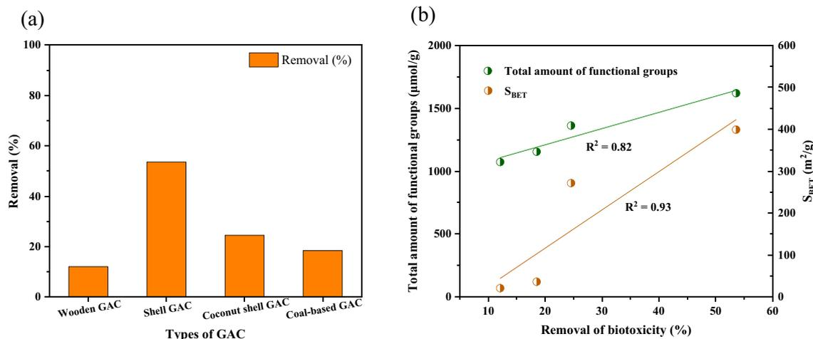
**Fig. 3.** The removal of the luminescent bacteria toxicity from SE using different GACs (a) and their relationship with the total amount of functional groups or  $S_{\text{BET}}$  (b).
