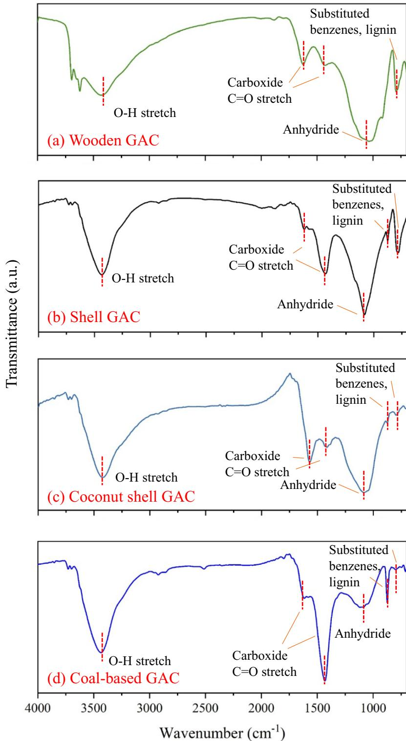
**Fig. 2.** FTIR spectra of four types of GACs. (a) Wooden GAC; (b) Shell GAC; (c) Coconut shell GAC; (d) Coal-based GAC.
